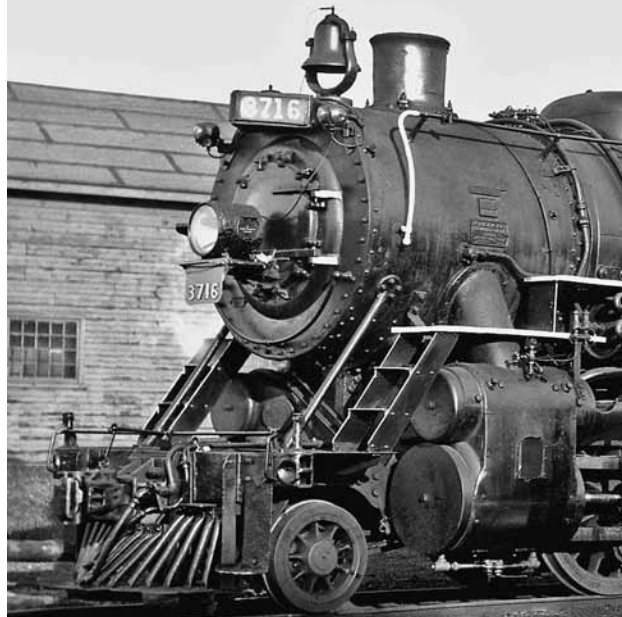
GT 3716, at Portland, Maine on March 3rd 1956, had the bell and road number lamp shifted to the top of the smokebox. When smaller-diameter headlights were installed on most GT and GTW locomotives, the support brackets remained unaltered. As a result, the headlights subsequently appeared to be off-centre – yet another trademark of “Trunk” lines in the USA. Those transferred permanently to Canada had their bracket centred and, with the larger rectangular CNR number plate, lost their “American” look. [PETER COX/DON McQUEEN COLLECTION]
